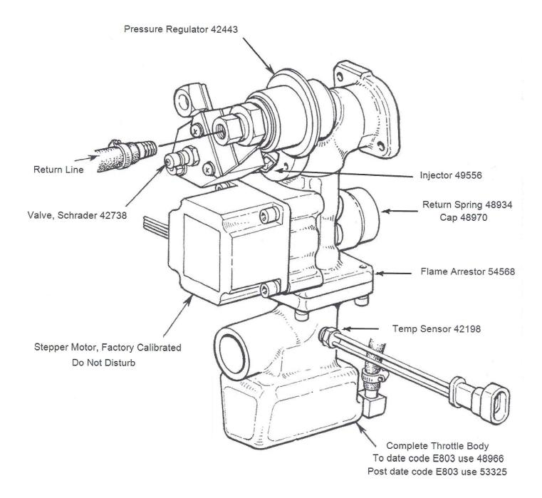
T-Body PN 48966 has a large bore throttle plate, it is used with ECU PN 49789.
